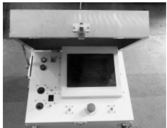
Fig. 14 Controller of cleaning device
