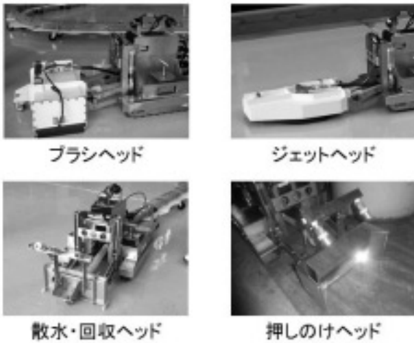
Fig. 9 Replaceable head tools of RACCOON II
