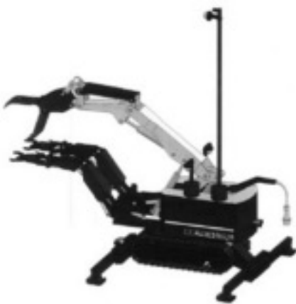
Fig. 12 Middle higher part decontamination equipment (dual-arm vehicle)
