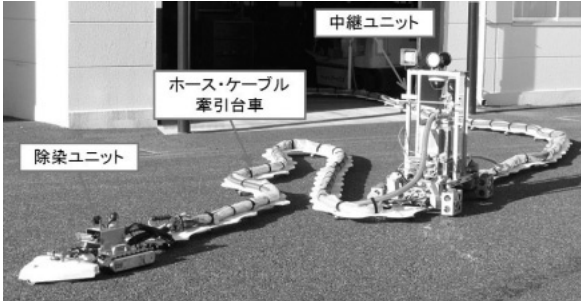
Fig. 5 Remote control compact decontamination robot, "RACCOON"
