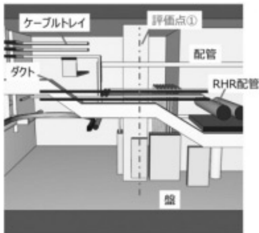
Fig. 20 Sample of radiation estimation model
